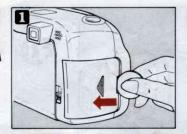
**2** Insert two 3V lithium batteries as shown and replace the cover. Use Panasonic CR123A, Duracell DL123A, or equivalent.
