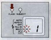
Use this mode in low light. If you use it in bright conditions, your picture will be overexposed. Use a tripod or other camera support to prevent the effects of camera shake. Press the PLASH button to set the This sectors of the USD provident of the sectors of the USD provident attain proper resolute. To prevent attain proper sectors are prevent attained processes resulting from catheres shales, the unread should be set formed in procure switters released
