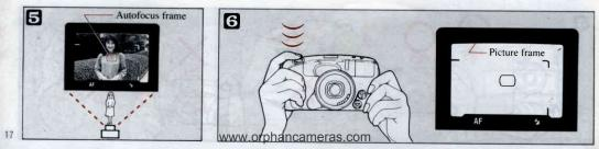
The entire subject should normally be positioned within the picture frame, however, the actual available image area will become smaller as you get hearer to the subject. At 0.6m(2ft), the subject should be positioned within the close-up correction marks. <sup>11</sup> S. Ger and elsent to most that W 53 and the platters' boost of the second second second results of the second sec
